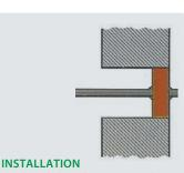
Finish and clean the opening edges then cut the panels with a cutters and position them in the opening. The edges and the jointing lines, as well as the interstices among the cables, are sealed and covered with FIRE STOP SEAL FSS sealant..
