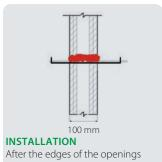
have been cleaned, shake the can for at least 30 seconds, then turn upside down and spray the product.
