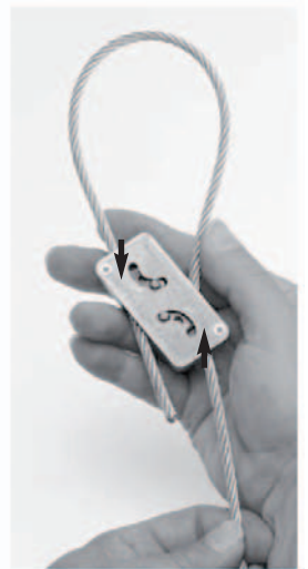
Step 5 To adjust, remove tension and pull wire rope slightly to disengage teeth, slide adjustment pin in direction shown by arrow to release wire rope
